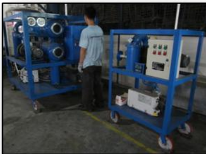
• Moisture Removal Equipment
